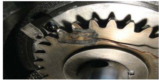
Fig.14 Previous simulations used thermocouple built in gear round the surface (left), concentrate at specific point at the surface (right).
